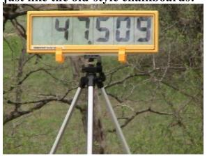
Each time any vehicle passes the IR Beam Transponder, the onboard Timer records the current lap time, instantly resets to zero and begins timing the next lap. The current lap ET is displayed on the trackside Big Display. Here are some examples:
