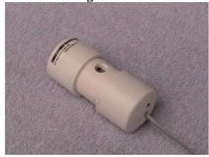
The IR Beam Transponder is located on the side of the track that the IR Beam Receivers on the vehicles will see when they pass. The Big Display is located where the driver can see his ET for the lap just completed – just like the old-style chalkboards!
